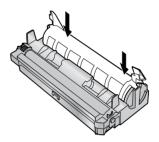
**5** Turn the two levers (①) on the toner cartridge firmly.
